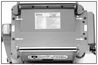
Figure 41. Feed roller lubrication points.
